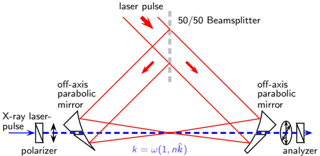
birefringence maximal for counter-propagating probe beam
