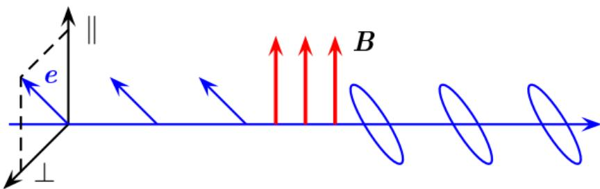
linear polarisation → elliptic polarisation
