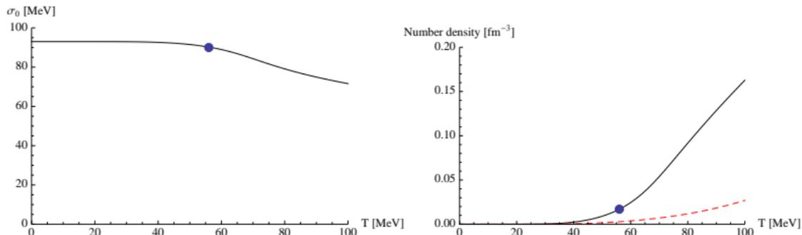
Left: Chiral condensate  $\sigma_0$  for  $\mu = 750 \text{ MeV}$ . The dot marks chemical freeze-out.
